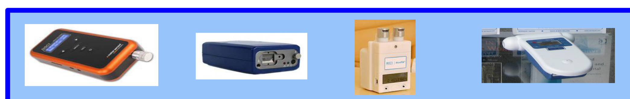
FIG 4. DISCMINI UFP, BC MICROAETH, PM2.5 MICROPEM, NO2 AEROQUAL SENSORS
